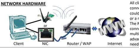
All clients need an NIC to connect to a ROUTER. This could be a wireless adapter or a network card. The Router in this simple connection can host multiple clients, but more advanced hardware is needed for bigger networks
