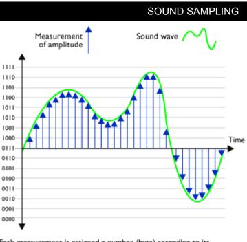
Each measurement is assigned a number (byte) according to its amplitude. The end result is a file comprising a string of bytes, eg ... 1001 1110 0001 1010 0111 0100 1111 1101 etc
