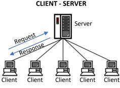
A single high-spec machine is designated the server, which includes the main file storage. Each client then *requests* data from the server which *responds* and fulfills the request.
